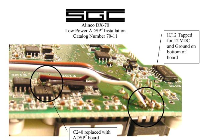
12 VDC can be taken from any point where it is convenient and the ground can be connected to any convenient point that is connected to the chassis ground. As shown in the picture, we chose to tap it from two pins on IC12.
